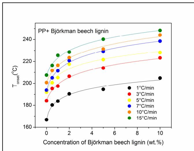
**Figure 11.** Thermal stability of polypropylene expressed as onset degradation temperature ( $T_{onset}$ ) in dependence on lignin concentration, heating scan 30 to 500°C, heating rate of 1, 3, 5, 7, 10 and 15 °C/min, oxygen flow (Gregorova et al., 2005a).
