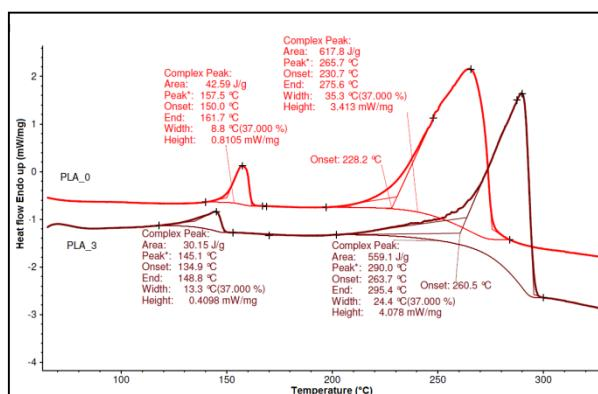
**Figure 10.** DSC curves of low molecular weight PLA synthetized by azeotropic dehydration condensation (PLA\_0) and modified by 2.5 mol.% succinic anhydride (PLA\_3), detected by 1<sup>st</sup> heating cycle from 30 to 350°C at heating rate of 10°C/min, in nitrogen flow.
