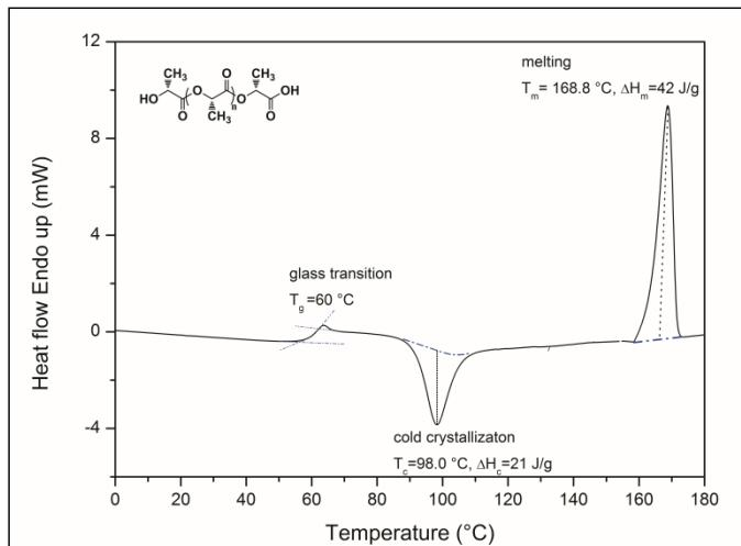
**Figure 1.** DSC thermogram of commercial poly(lactic acid) with  $M_w = 70\,400$  and PDI = 1.8 detected during 2<sup>nd</sup> heating cycle (0–180°C, 10°C/min, N<sub>2</sub> atmosphere)
