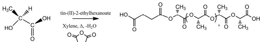
**Figure 7.** Structure of PLA<sub>3</sub> (PLA synthesized by the azeotropic dehydration condensation and modified by 2.5 mol% succinic anhydride)
