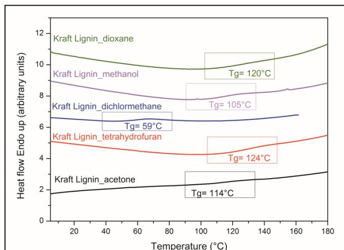
**Figure 4.** DSC thermograms of Kraft lignin extracted in acetone, tetrahydrofuran, dichlormethane, methanol and 1,4-dioxane detected during second heating scan (5-180°C, 10°C/min, N<sub>2</sub> atmosphere)
