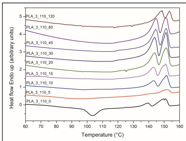
**Figure 8.** DSC thermograms of PLA<sub>3</sub> annealed at 110°C for 0-120 min (1<sup>st</sup> heating, 30-160°C, 10°C/min, N<sub>2</sub> atmosphere)
