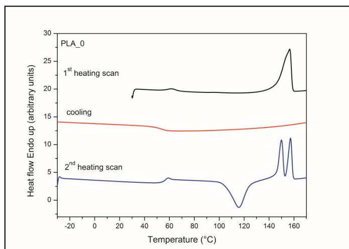
**Figure 5.** DSC thermogram of PLA\_0 detected during heating/cooling/heating scan (30-170°C, 170-0°C, -30-170°C, 10°C/min, N<sub>2</sub> atmosphere)
