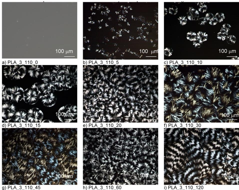
**Figure 9.** Polarized optical micrographs (magnification 400 $\times$ ) of crystals of polylactic acid modified with succinic anhydride (PLA\_3) grown from the melt and annealed at 110°C for 5-120 min
