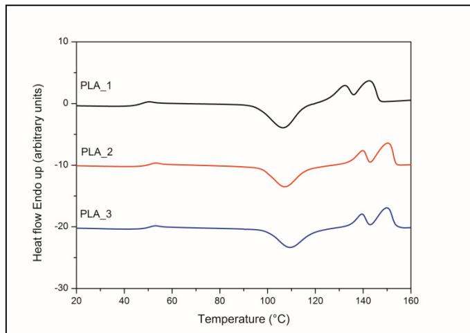
**Figure 6.** DSC thermograms of PLA samples with modified side chain groups and various molecular properties detected during second heating scan (-30-170°C, 10°C/min, N<sub>2</sub> atmosphere)
