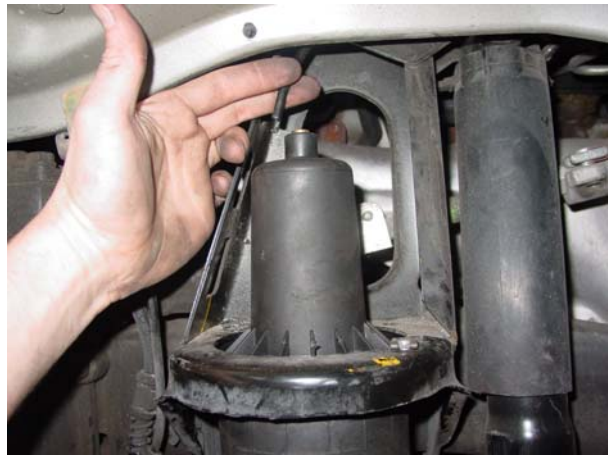
4. Depressurize air spring by removing nylon air hose. To remove air hose, push down on the metal collet, while pulling out on the hose. ↑
