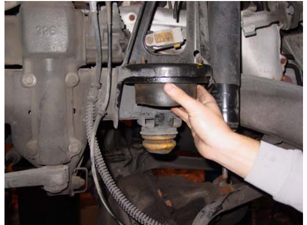
10. Install upper coil spring rubber isolator. ↑
